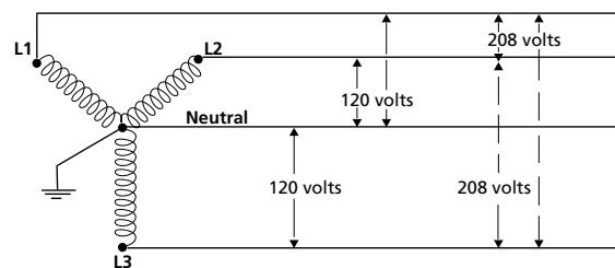
A Delta PDU would use a NEMA L21-30P (the mating Wye plug), but would not use a neutral inside the PDU. This is a perfectly acceptable practice. For example, a data center could deploy Delta PDUs to racks where there is only a need for 208V and Wye PDUs to racks where there is a need for both 120V and 208V.
