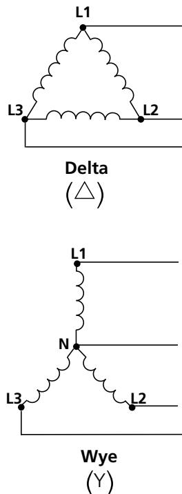
Since the difference between Delta and Wye is whether or not there is a neutral, many data centers are wired for Wye and use whips terminated with Wye receptacles such as NEMA L21-30R. This means the data center can use Wye PDUs which support 120V/208V or use Delta PDUs which support only 208V without needing to change the data center wiring.
