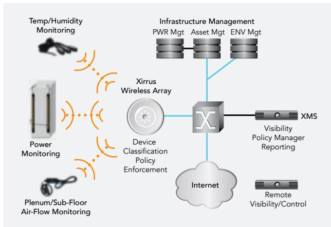
Once properly deployed, a comprehensive DCIM solution provides data center operations managers with clear visibility of all data center assets along with their connectivity and system status. However, along with the advantages of this new approach come challenges, specifically how to interconnect all the intelligent monitoring and control devices.
