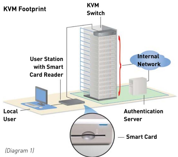
The components mentioned in Diagram 1 are part of the KVM footprint. On the server side, special middleware deployed on each target server communicates with the card reader and the authentication infrastructure that’s in place. The middleware is essentially a “go-between” that utilizes various specifications (such as PC/SC and x.509) and support PKI certificates – enabling the use of smart cards for a wide variety of desktop, network security and productivity applications.
